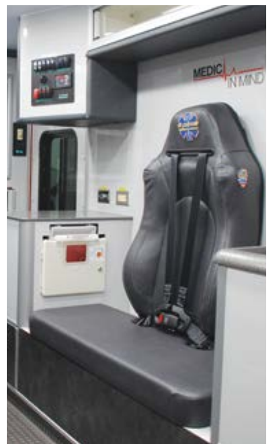
Optional Medic in Mind with Valor Backrest 4 point restraint with 4 retractors and single release buckle
